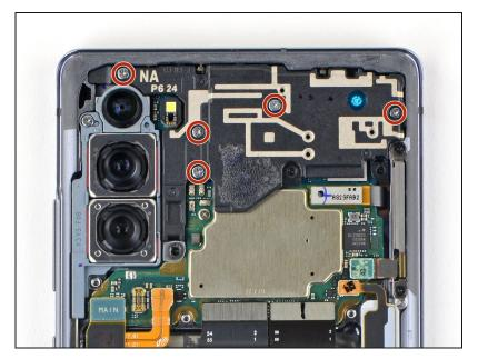
Use a Phillips screwdriver to remove the five 4.0 mm screws securing the earpiece speaker to the frame.
