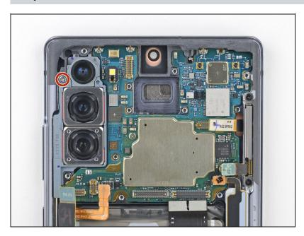
Use a Phillips screwdriver to remove the 4.0 mm screw securing the motherboard to the frame.
