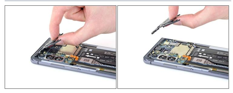
Lift and remove the earpiece speaker.
