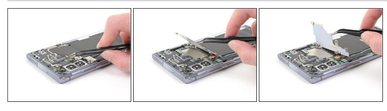
Use a pair of tweezers to lift up and flip back the motherboard shield.
