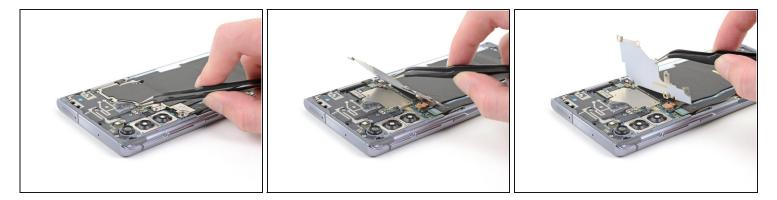
• Use a pair of tweezers to lift up and flip back the motherboard shield.
