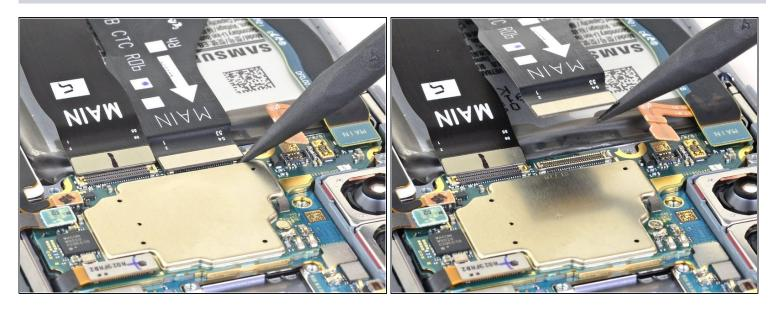
• Use the pointed end of a spudger to disconnect the main interconnect cable from the motherboard.
