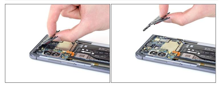
• Lift and remove the earpiece speaker.
