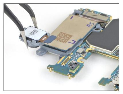
• Use a pair of tweezers to lift and remove the upper camera from the motherboard.
