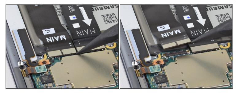
• Use the pointed end of a spudger to disconnect the display cable from the motherboard.
