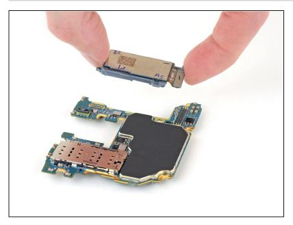
• Lift and remove the lower cameras from the motherboard.
