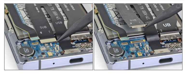
• Use the pointed end of a spudger to disconnect the main interconnect cable from the daughterboard.
