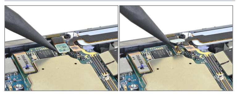
• Use the pointed end of a spudger to disconnect the green press connector from the motherboard.
