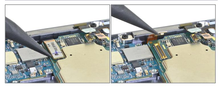
• Use the pointed end of a spudger to disconnect the touch layer press connector from the motherboard.
