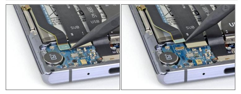
• Use the pointed end of a spudger to disconnect the secondary interconnect cable from the daughterboard.
