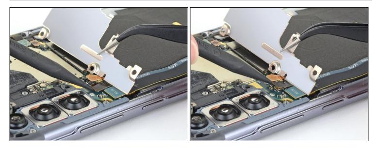
• While using a pair of tweezers to hold the motherboard shield out of the way, use the pointed end of a spudger to pry up the wireless charging coil press connector.
