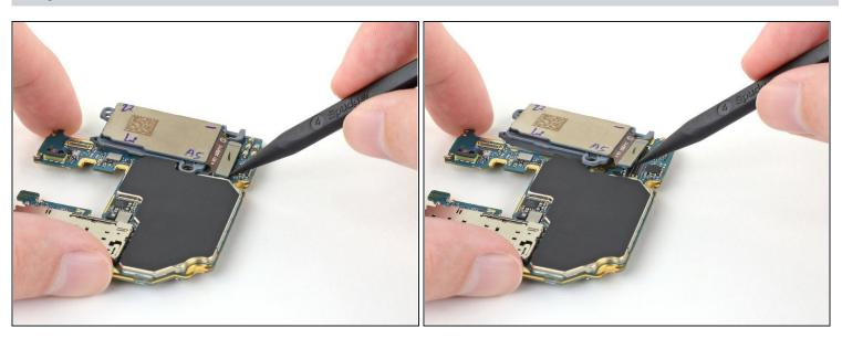
• Use the pointed end of a spudger to pry up the lower cameras' press connector from the motherboard.
