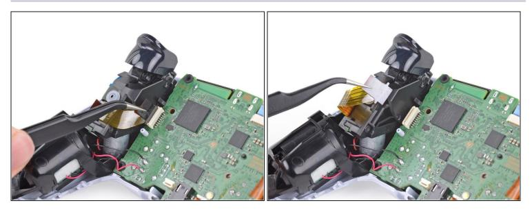
Grip the right trigger assembly ribbon cable pull tab with a pair of tweezers or your fingers and pull up to disconnect it from the motherboard.
