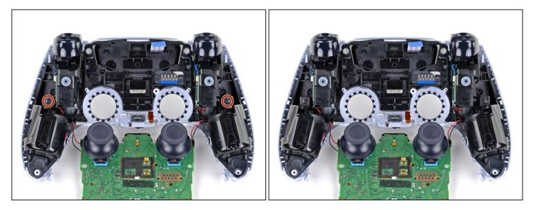
• Use a Phillips screwdriver to remove the two 6.4 mm screws securing the midframe to the front case.
