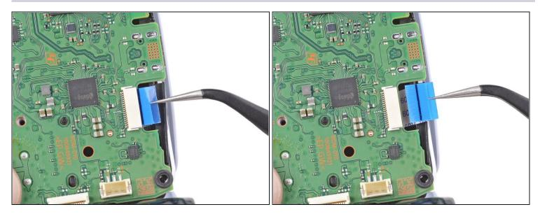
• Use a pair of tweezers or your fingers to grip the touchpad ribbon cable pull tab, and pull it straight out of the motherboard connector.
