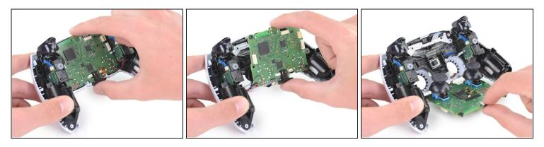
• Carefully guide the joysticks through the front case and lift the motherboard out.
