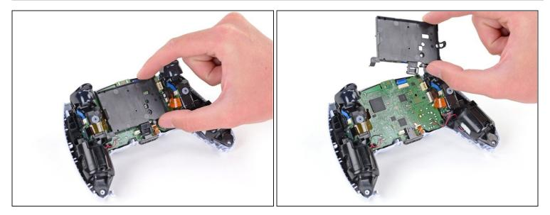
• Lift the battery bracket out of the motherboard.
