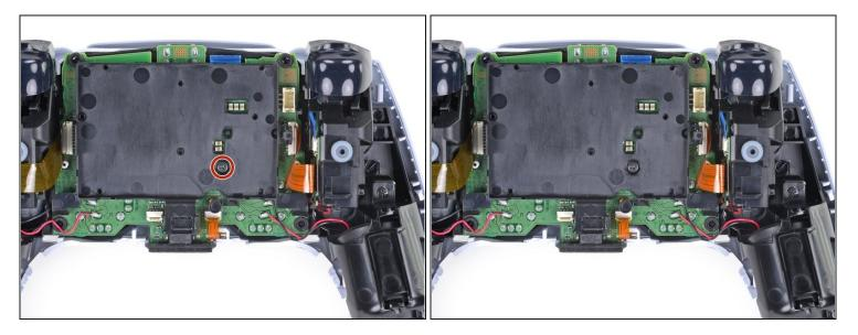
• Use a Phillips screwdriver to remove the 6.4 mm screw securing the battery bracket.
