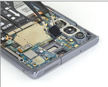
Use a pair of tweezers to remove the front-facing camera.
