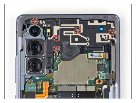
Use a Phillips screwdriver to remove the five 4.0 mm screws securing the earpiece speaker to the frame.
