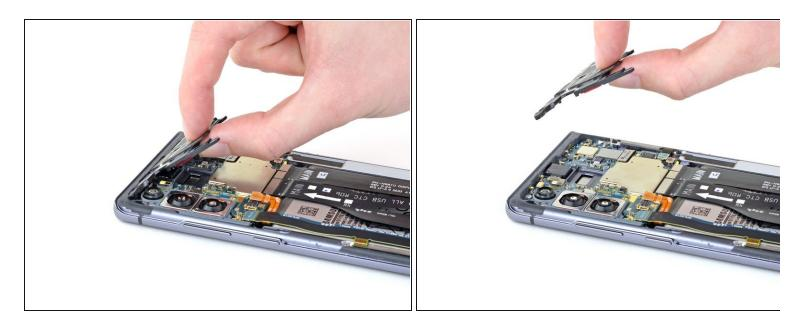
• Lift and remove the earpiece speaker.
