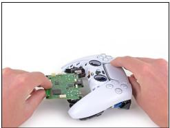
• Carefully flip over the controller and motherboard.
