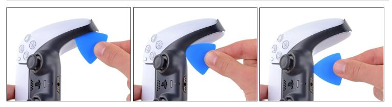
• Slide the opening pick along the lower-right edge of the middle trim to release the clips securing it to the case.
