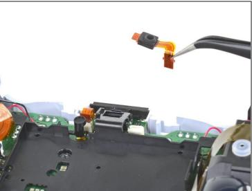
• Grab the lower microphone ribbon cable pull tab with your fingers or a pair of tweezers and disconnect it from the motherboard.
