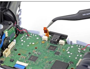
• Use a pair of tweezers or your fingers to grip the upper microphone ribbon cable pull tab, and pull up to disconnect it from the motherboard.
