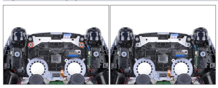
• Use a Phillips screwdriver to remove the two 8.5 mm screws securing the light guide.
