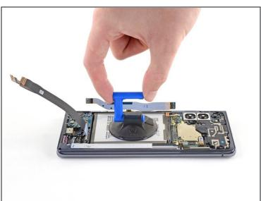
• Apply a suction cup to the center of the battery.
