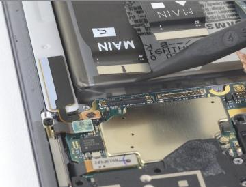
• Use the pointed end of a spudger to disconnect the display cable from the motherboard.
