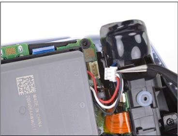
Use a pair of tweezers or your fingers to disconnect the battery from the motherboard.
