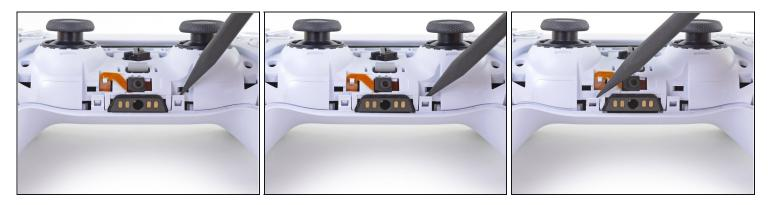
• Use the pointed edge of a spudger to unclip the two clips on either side of the headset jack.
