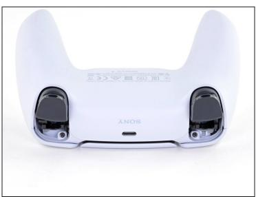
• Use a Phillips screwdriver to remove the two 6.4 mm screws behind the **L1** and **R1** buttons.
