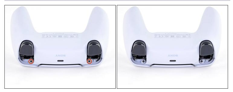
• Use a Phillips screwdriver to remove the two 6.4 mm screws behind the **L1** and **R1** buttons.
