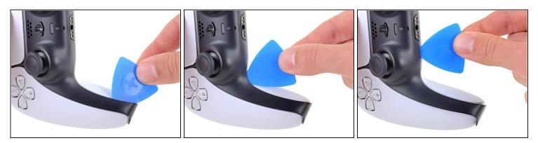
• Slide the opening pick along the lower-left edge of the middle trim to release the clips securing it to the case.
