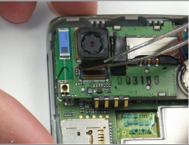
Locate the camera near the upper-left corner and use the metal tweezers to carefully detach the black tab.
