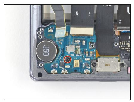
Use a Phillips screwdriver to remove the 2.9 mm screw securing the daughterboard to the frame.
