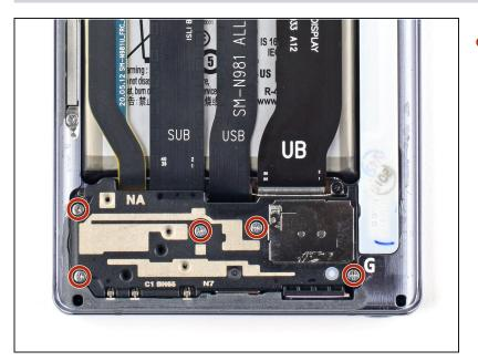
Use a Phillips screwdriver to unscrew the five 4.0 mm screws securing the loudspeaker to the frame.
