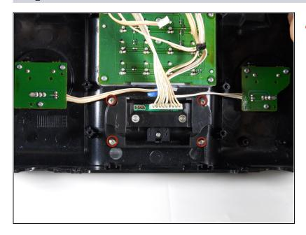
• Remove the four 6.4 mm Phillips #1 screws holding the adapter to the outer case.
