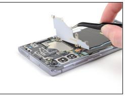
Use a pair of tweezers to lift up and flip back the motherboard shield.
