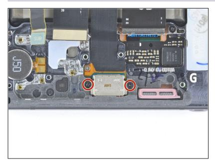
Use a Phillips screwdriver to remove the two 2.9 mm screws securing the USB-C port to the phone.
