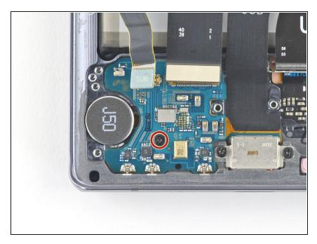
• Use a Phillips screwdriver to remove the 2.9 mm screw securing the daughterboard to the frame.
