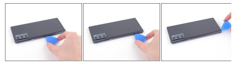
As you cut through the adhesive around the perimeter of the phone, don't insert the pick more than 5 mm to avoid damaging internal components.
