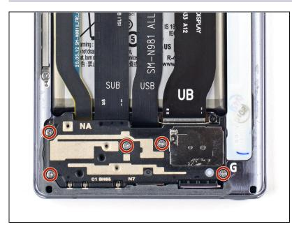
Use a Phillips screwdriver to unscrew the five 4.0 mm screws securing the loudspeaker to the frame.
