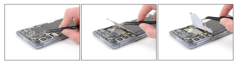
Use a pair of <u>tweezers</u> to lift up and flip back the motherboard shield.
