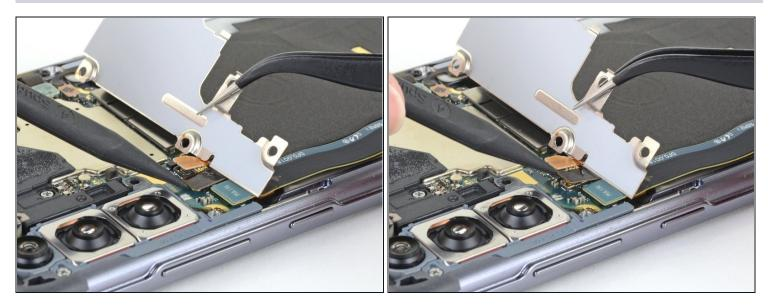
• While using a pair of tweezers to hold the motherboard shield out of the way, use the pointed end of a spudger to pry up the wireless charging coil press connector.
