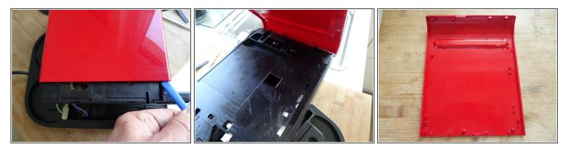
• The two colored side panels are only snapped into place. However, the latches sit very tight. You really need a lot of force. First lift the lower edge using a plastic opening tool.
