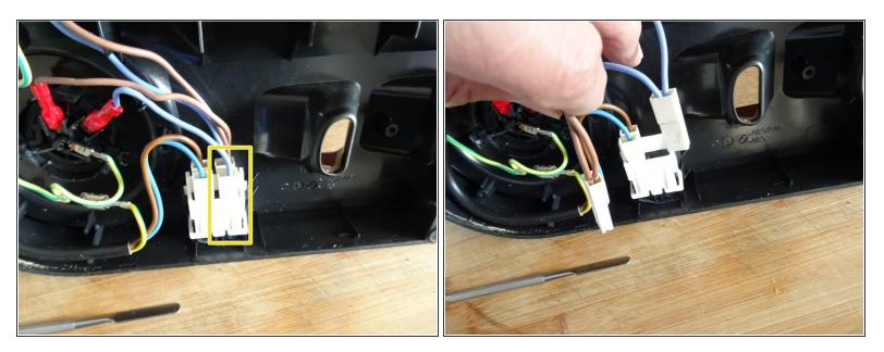
Disconnect the two spade plugs on the blue and brown wires from the power switch. The two left ones remain.
