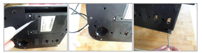
The bottom panel is just snapped into place. Insert a metal spudger into the slots and lift the panel out. It sits quite tightly and you might use some force to get it out.
