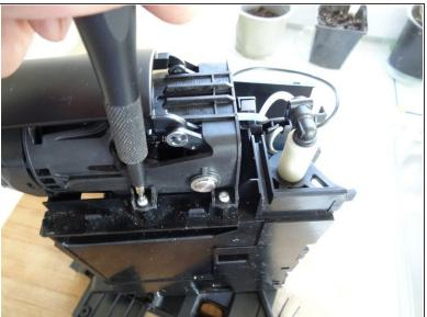
Use a Torx T10 screwdriver to remove the four screws securing the brewing unit.
