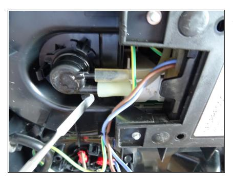
Use a spudger to slide off the two silicon tubes.
