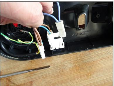
Disconnect the two spade plugs on the blue and brown wires from the power switch. The two left ones remain.
