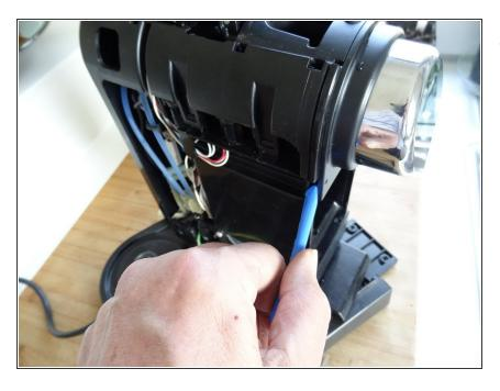
Insert a opening tool in the gap on the bottom of the coffee spout. Pry it off carefully.
