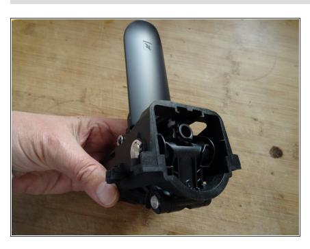
Lift the brewing unit from the device.
