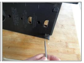
The bottom panel is just snapped into place. Insert a metal spudger into the slots and lift the panel out. It sits quite tightly and you might use some force to get it out.
