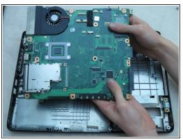
• Gently lift the top right side of the motherboard. Pull it upwards to the right and away from you.
