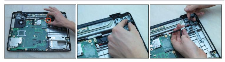
• Using your fingers, gently slide the heading with two black wires and two red wires out of its receptacle. Gently slide the power jack up.
