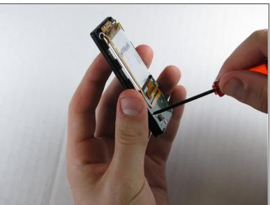
Remove the three screws (5.5mm by 3mm) from the backside of the Zune using a small Tri-Wing screwdriver.
