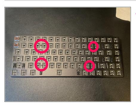
Use a # 1 philips drill bit to remove the 4 screws on the keyboard
