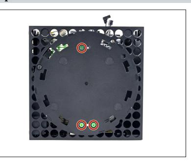
Use a T8 Torx driver to remove the three 7.4 mm screws securing the center chassis assembly to the shell.
