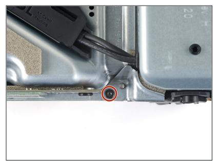
Use a T8 Torx driver to remove the 8.8 mm screw securing the power supply corner cover.
