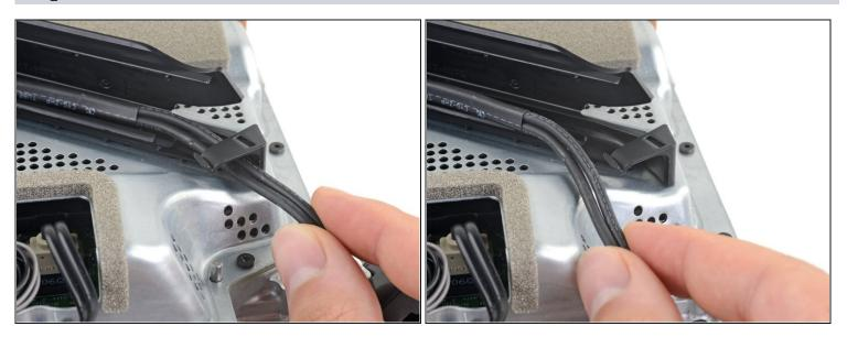
• Lift the power cable out from underneath the extra section of the cable guide.
