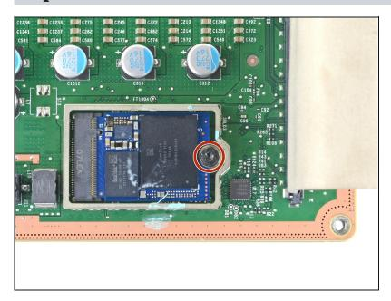
Use a T8 Torx driver to remove the 5.2 mm screw securing the SSD.
