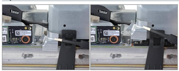
• Use your fingers or a pair of <u>tweezers</u> to lift and remove the power supply corner cover.
