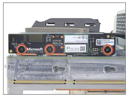
• Use a T8 Torx driver to remove the three 9.6 mm screws securing the accessory antenna board to the center chassis.
