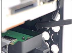
• Use the flat end of a spudger to lift up on the locking tab holding the base to the shell.
