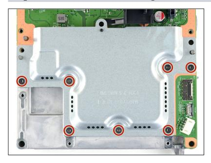
Use a T8 Torx driver to remove the seven 8.8 mm screws securing the southbridge board shield.
