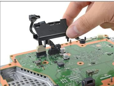
• Lift up to remove the power supply cable guide from the southbridge board.
