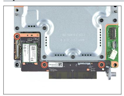
Use a T8 Torx driver to remove the three 8.8 mm screws securing the Wi-Fi antenna board.
