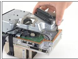
• Lift up the board shield to remove it from the center chassis.
