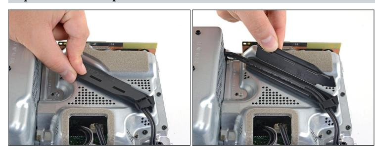
• Unlatch and open the lid on the power cable's plastic guide.
