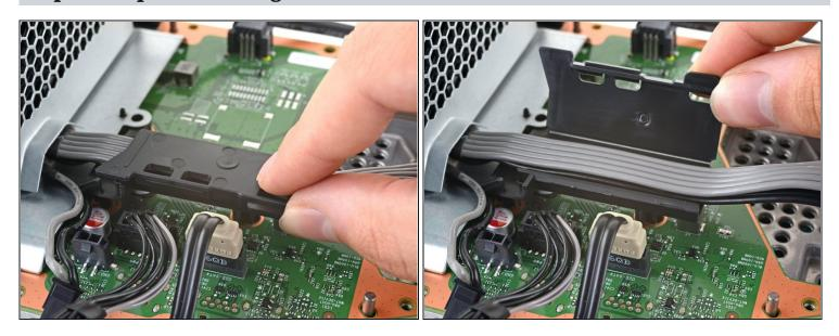
• Open the lid on the power supply's plastic cable guide.
