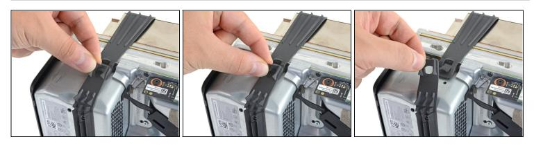
• Unlatch the chassis strap from the right side of the power supply.
