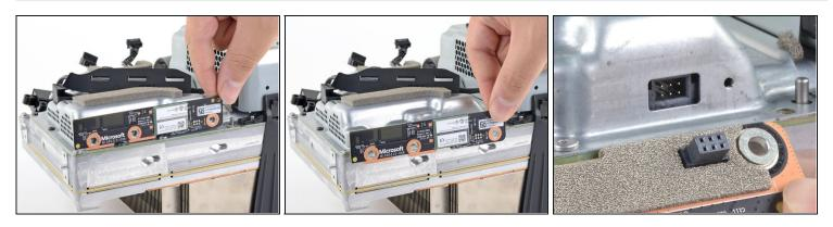
• Grip the antenna board and pull it directly away from the center chassis to disconnect it.
