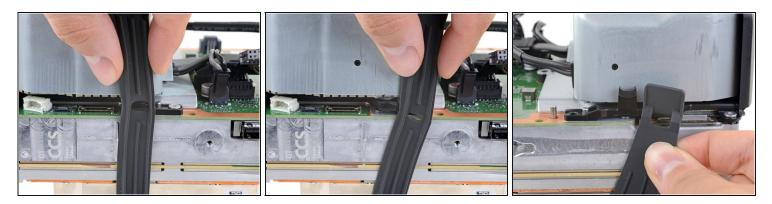
• Disconnect the chassis strap from the locking tabs on either side of the power supply.
