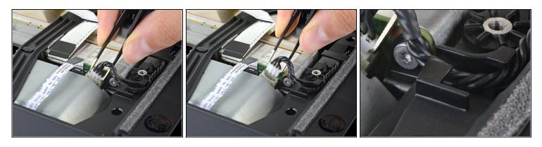
Use your fingers or a pair of blunt tweezers to grip the edges of the fan cable connector, and pull up to disconnect it from the center chassis.
