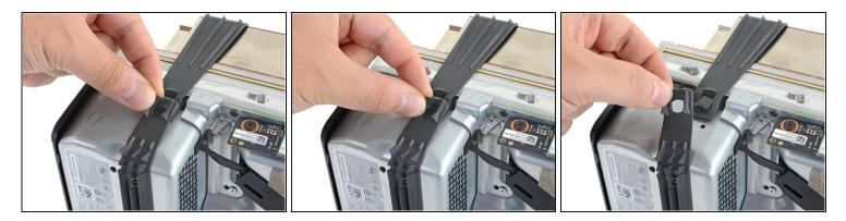
• Unlatch the chassis strap from the right side of the power supply.
