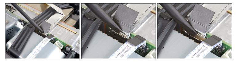
The ribbon cables and their connectors are extremely fragile, so always open locking tabs gently and pull cables slowly.
