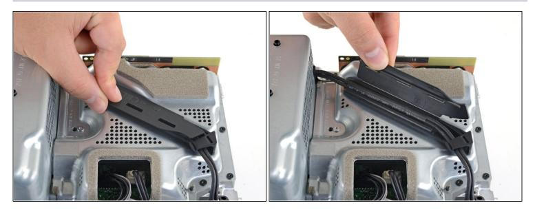
• Unlatch and open the lid on the power cable's plastic guide.
