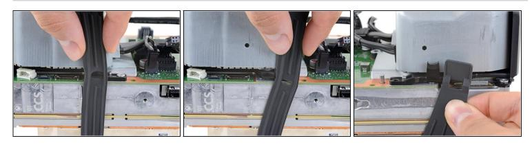
Disconnect the chassis strap from the locking tabs on either side of the power supply.
