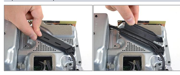
Unlatch and open the lid on the power cable's plastic guide.
