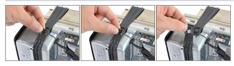
• Unlatch the chassis strap from the right side of the power supply.
