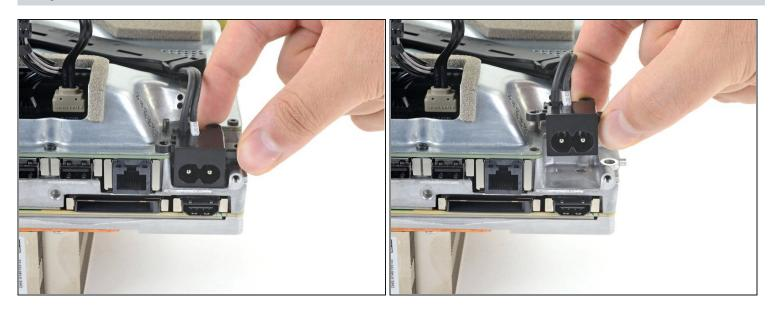
• Lift the power connector out of its recess in the chassis.
