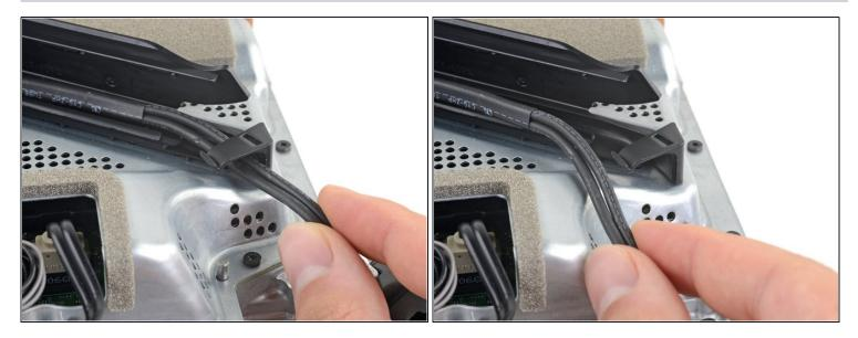
• Lift the power cable out from underneath the extra section of the cable guide.
