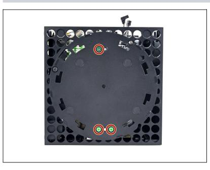
Use a T8 Torx driver to remove the three 7.4 mm screws securing the center chassis assembly to the shell.
