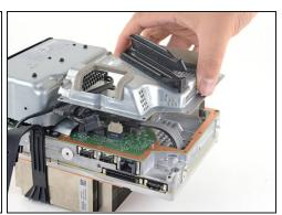
Lift up the board shield to remove it from the center chassis.
