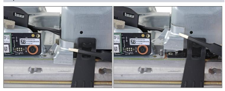
• Use your fingers or a pair of tweezers to lift and remove the power supply corner cover.
