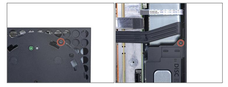
Use a T8 Torx driver to remove the two 8.8 mm screws securing the optical drive's vibration isolator to the shell: one on the base and one on the top of the isolator.
