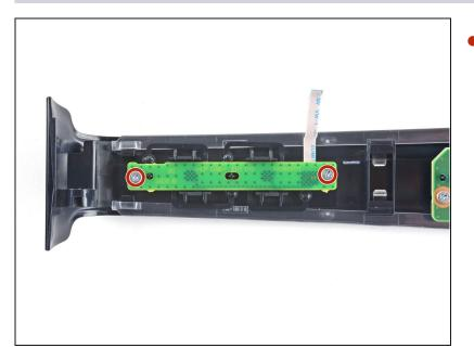
• Use a Phillips screwdriver to remove the two 6.5 mm-long screws securing the power and eject button board to the middle panel.
