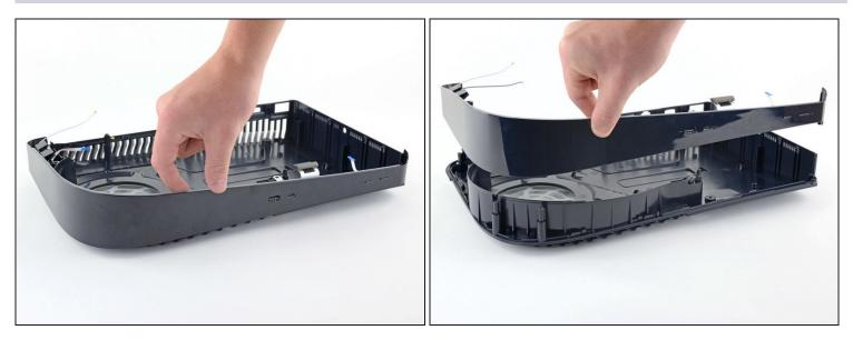
• Lift up to remove the middle panel from the case.
