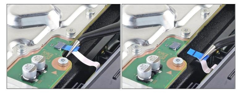
• Use a pair of tweezers to pull the blue pull tab directly away from the connector to disconnect the power and eject button ribbon cable.
