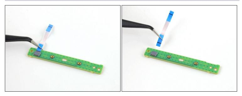
• Use a pair of tweezers to pull the blue pull tab directly away from the connector to disconnect the power and eject button ribbon cable.
