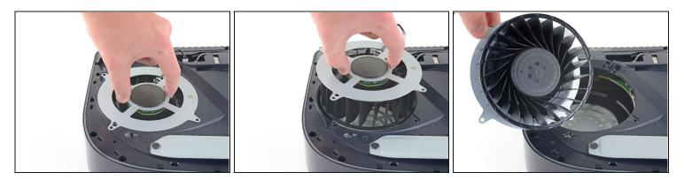
• Lift the fan up and out of the case to remove it.
