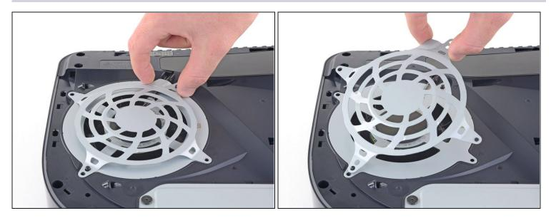
• Lift the fan shroud straight up to remove it.
