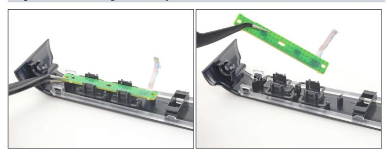
• Use a pair of tweezers to remove the power and eject button board from the middle panel.
