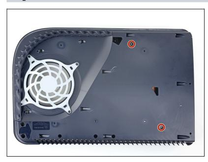
Use a Torx T8 driver to remove the two 29.4 mm-long screws securing the case to the motherboard and heat sink assembly.
