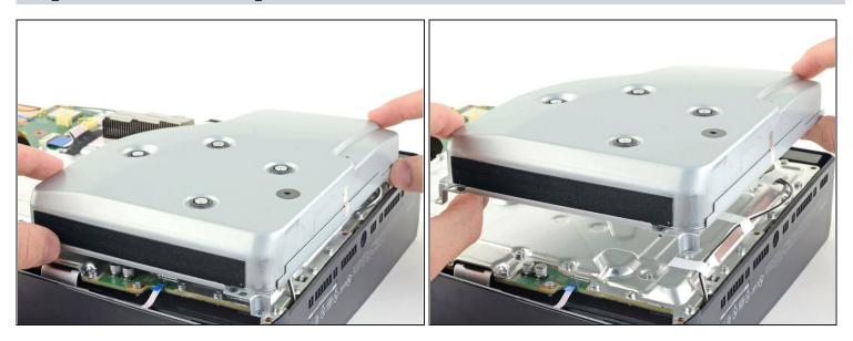
• Lift the optical drive away from the device to remove it.
