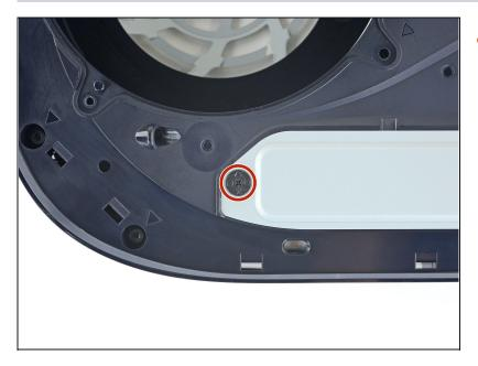
Use a Phillips screwdriver to remove the 17 mm-long SSD cover screw.
