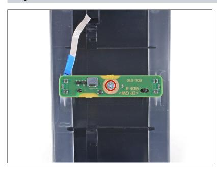
Use a Phillips screwdriver to remove the 6.5 mm-long screw securing the LED board to the middle panel.
