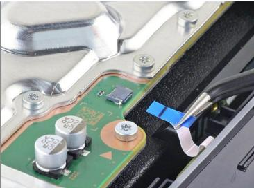
• Use a pair of tweezers to pull the blue pull tab directly away from the connector to disconnect the power and eject button ribbon cable.
