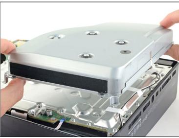
Lift the optical drive away from the device to remove it.
