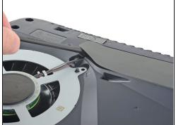
• Insert the flat end of a spudger beneath the black wire cover and into the gap above the fan wires.
