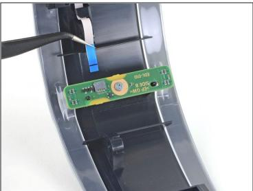
• Use a pair of tweezers to pull the blue pull tab directly away from the connector to disconnect the LED board ribbon cable.
