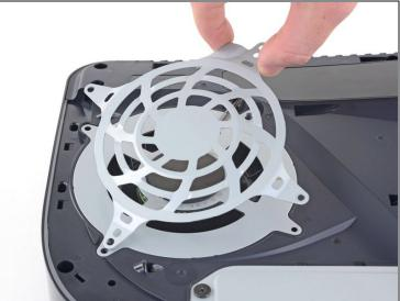
• Lift the fan shroud straight up to remove it.
