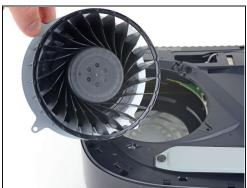
• Lift the fan up and out of the case to remove it.
