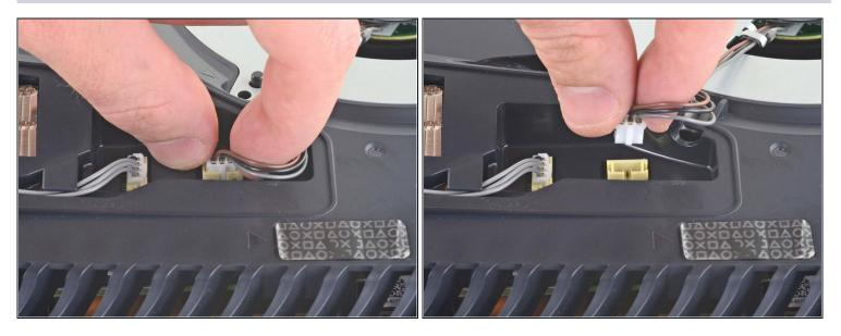
• Use your fingers to grip the edges of the fan cable connector, and pull up to disconnect it from the motherboard.
