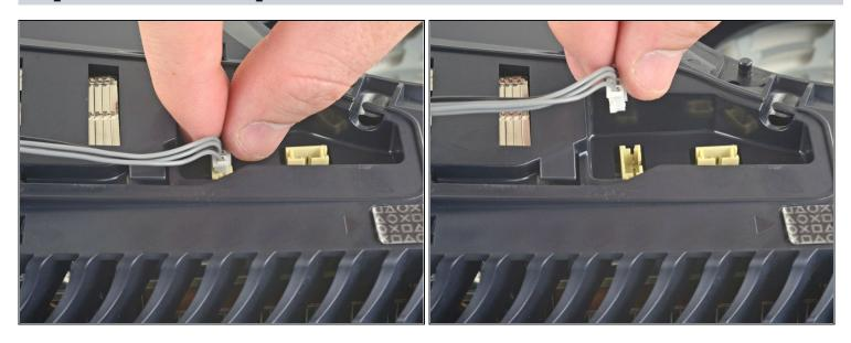
• Use your fingers to grip the edges of the optical drive cable connector, and pull up to disconnect it from the motherboard.
