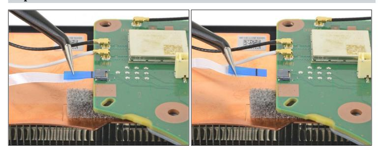
• Use a pair of tweezers to pull the blue pull tab directly away from the connector to disconnect the LED ribbon cable.
