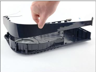
• Lift up to remove the middle panel from the case.
