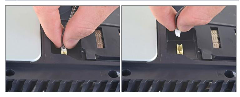
Use your fingers to grip the edges of the optical drive cable connector, and pull up to disconnect it from the optical drive.
