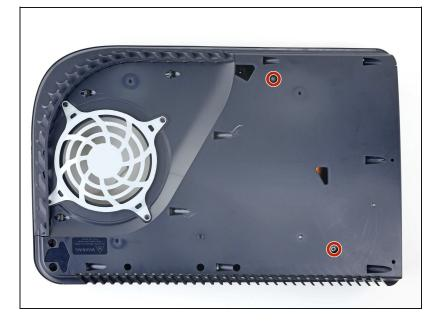
Use a Torx T8 driver to remove the two 29.4 mm-long screws securing the case to the motherboard and heat sink assembly.
