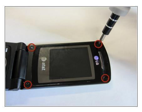
Remove the four 3 mm Phillips #00 screws.
