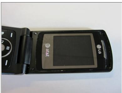
Use an opening tool to remove the thin silver part covering the speaker at the top of the phone.
