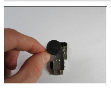
Pull speaker out of the component by grabbing the wire attached to it in order to replace it.
