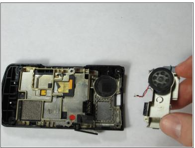
Remove the speaker component from the back of the phone by lifting up the top part to a 45 degree angle and pulling it out.
