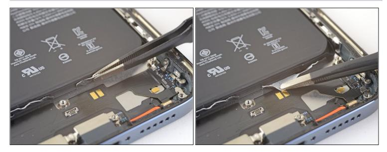
• Peel down the second battery adhesive pull-tab to un-stick it from the bottom edge of the battery.
