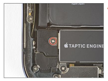
• Use a Phillips driver to remove the 1.4 mm screw securing the Taptic Engine plastic cover.
