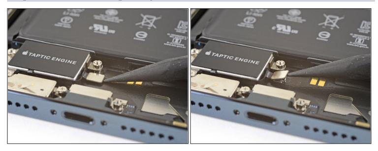
• Use the point of a spudger to pry the Taptic Engine connector straight up and out of its socket.
