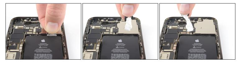
• Using the same procedure as before, pull the remaining two tabs, one at a time, to stretch and remove the remaining adhesive strip holding the battery in place. Try not to snag the adhesive on anything.
