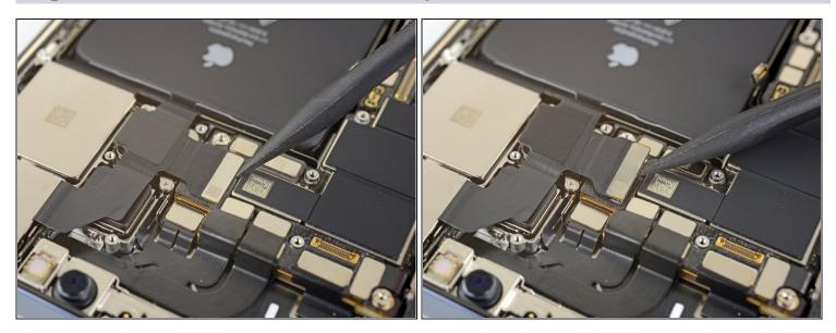
• Use a spudger or a fingernail to disconnect the first camera cable connector by prying it straight up from its socket.
