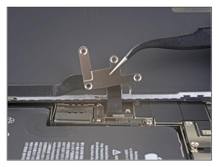
• Remove the battery and display connector cover.
