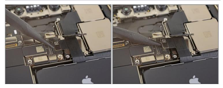
• Use a spudger or a fingernail to disconnect the second camera cable connector by prying it straight up from its socket.
