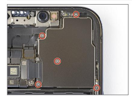
Use a Y000 driver to remove the five 1.5 mm screws securing the rear-facing camera cover.
