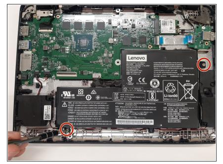
Using the Phillips #0 screwdriver, remove the two 3 mm screws holding the battery in place.
