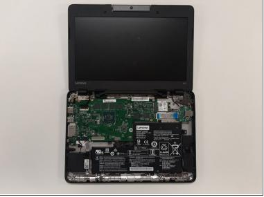
Lift the keyboard panel from the case and fully remove it from the device.
