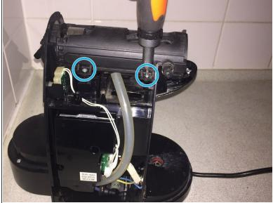
• Use a Torx T10 ro remove the 4 screws that hold the the brew unit, 2 on each side.
