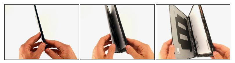
• Open the display casing along the top edge.
