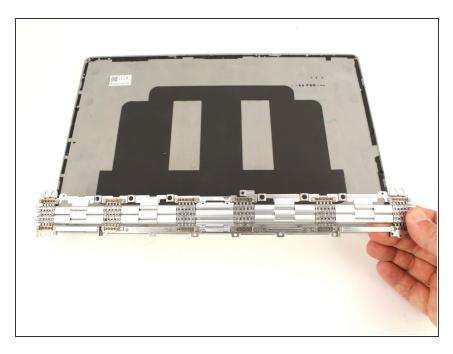
• Lift off the hinge assembly.
