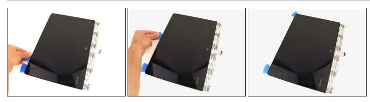
• Continue cutting away the adhesive on the top and side edges of the display.
