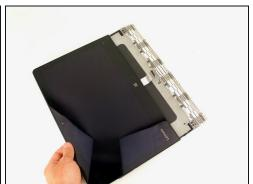
Pull the display cable out from the hinge mechanism.
