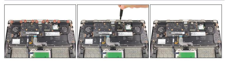
• Remove the ten 3.6 mm screws from the hinge bracket with a Phillips #00 screwdriver.
