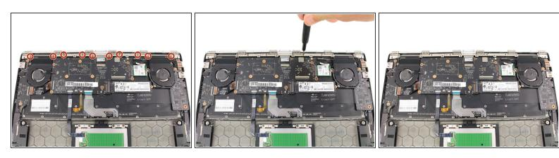
Remove the ten 3.6 mm screws from the hinge bracket with a Phillips #00 screwdriver.
