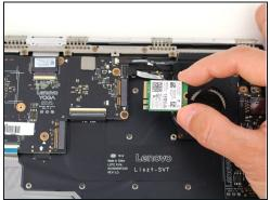
• Pull the WiFi card out from the connector on the motherboard.
