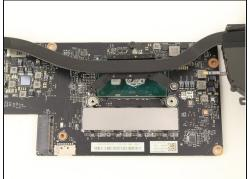
• Unscrew the three captive screws on the heatsink with a Phillips #1 screwdriver.
