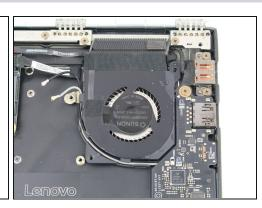
• Remove the two 3.6 mm screws from the right fan using a Phillips #00 screwdriver.
