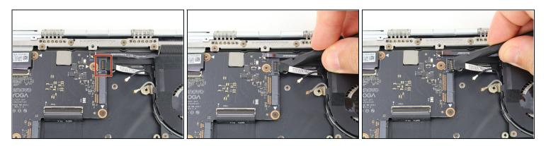
• Use a spudger to pry up the <u>press fit connector</u> on the right side of the motherboard.
