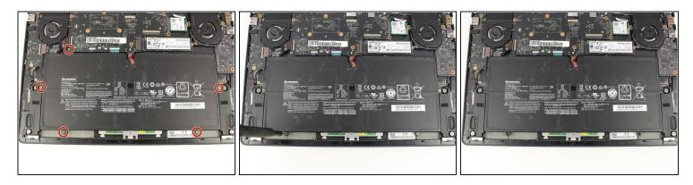
• Remove the five 3.6 mm screws from the battery with a Phillips #00 screwdriver.
