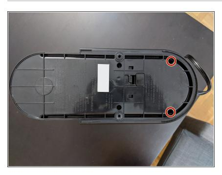
Remove two phillips screws on the base.
