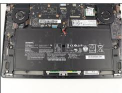
• Remove the five 3.6 mm screws from the battery with a Phillips #00 screwdriver.
