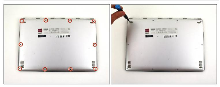
• Using a T5 Torx screwdriver, remove the ten 5.5 mm screws from the back case of the laptop.
