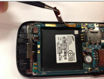
• Use the tweezers to unclip the orange ribbon cable from the left side of the phone.
