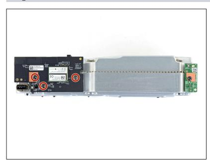
Use a T8 Torx driver to remove the three 9.5 mm-long screws securing the Bluetooth board to the long edge of the chassis.
