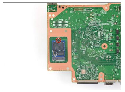
Use a T8 Torx driver to remove the 5.1 mm-long screw securing the SSD card to the motherboard.
