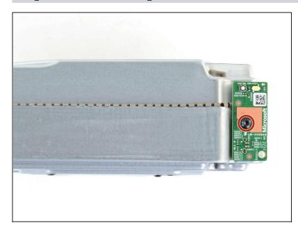
• Use a T8 Torx driver to remove the 9.5 mm-long screw securing the power button board to the chassis.
