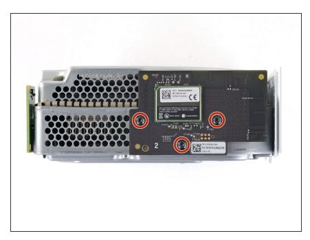
Use a T8 Torx driver to remove the three 9.5 mm-long screws securing the Wi-Fi board to the short edge of the chassis.
