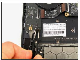
Use a pair of blunt nose tweezers or your fingers to pull out the speaker cable from the connector on the lower portion of the daughterboard.
