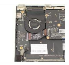
Using a Phillips #00 screwdriver, remove the two 3.6 mm screws from the daughterboard.
