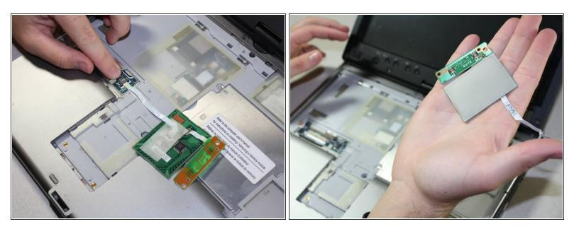
Pull back the tab to disconnect the touchpad to the laptop.
