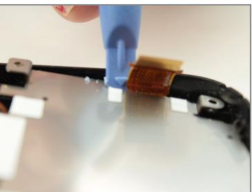
• Insert plastic opening tool as shown and lift up to dislodge plate from tab.
