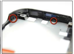
• Locate the four tabs above the keyboard. The following steps will demonstrate how to remove the metal plate from the tabs, which will reveal the keyboard.
