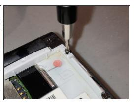
Now we will remove the first screws. You will need a T5 Torx screwdriver or screwdriver bit to remove the four screws on the back. One of the screws is hidden underneath a black plastic circle, remove that.
