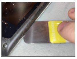
• Phew! We've done a lot of work on the bottom of the phone. Let's go to the top with the screen! First, use tweezers to remove the yellow rubber coverings over the screws, then use your T5 Torx driver to remove all four screws. Now work your way around the screen edge with an opening tool, then lift the cover!
