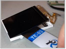
Now, the moment we've been waiting for... THE MAIN SCREEN REMOVAL! Carefully lift the screen circuit board out, unlatch the two white clips and carefully lift the screen backlight off. Now remove the metal cover on the back of the screen, remove the glued-on wire, and ever so carefully, use an opening tool to go UNDER the screen and boom! It's off!
