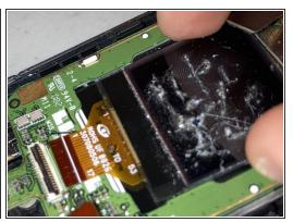
• Wow! There sure are a lot of connections to the screen! Let's remove them! Use tweezers to lift the metal connector, lift the black lever on the plastic connectors and pull out the wires, and lift the maroon plastic connector. The two black plastic connectors connect the small front screen and the camera, so you will remove these after the wires.
