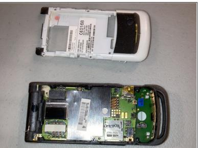
Now to the fun part, opening the phone! Use an opening tool and work your way around the edges of the back cover. Then lift it and we're in!
