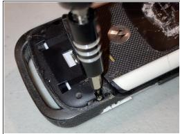
• After the first screws are removed, let's take a look at the front. On the bottom of the front, there is a plastic cover blocking two screws. Work your way around the edges of the cover with an opening tool to remove it, then lift the cover and remove the two remaining external Torx screws.
