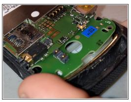
Now back to the phone. We are now at the circuit board. There is one connection to the screen on the back of the board (see pictures). We need to separate it from the board. Use tweezers to carefully lift the click connector. Next, there are two clips on the board. Use tweezers to push one in, then push the other in and lift the board.
