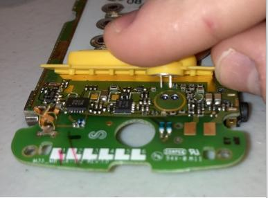
• If we flip over the board, there are some removable parts. 1: The rubber keypad buttons. Simply pull them off as they are only glued a little. 2: The phone call mic. Pull up on the little yellow strip of rubber to remove. Don't panic when you see the bottom of the mic, it looks like you pulled out the soldering, but you didn't, just a connector!
