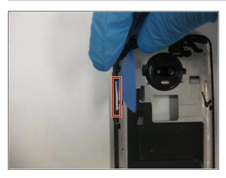
Use the pick to pry off the white plastic piece that holds the volume and power buttons in place.
