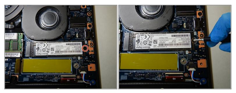
• Using the Phillips #00 screwdriver, remove the single screw securing the SSD to the motherboard.
