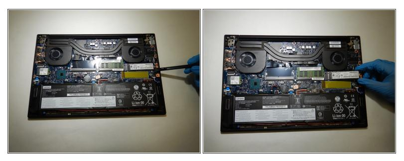
Using the opening tool, pop out the SSD card and remove it from the device.
